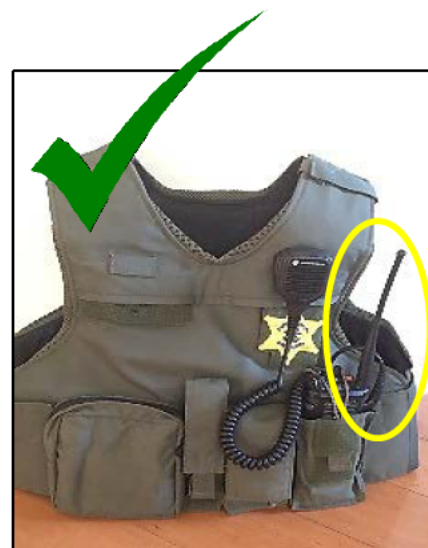
The antenna SHOULD be free from any obstructions and the radio holstered or held in an upward position.
